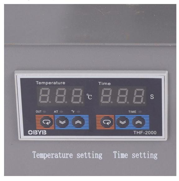
1, Press the " $\bigcirc$ " button to set the temperature (the default setting is 287°C). Adjust the temperature using the " $\approx$ " or " $\approx$ " buttons, and press the " $\bigcirc$ " button to confirm.
