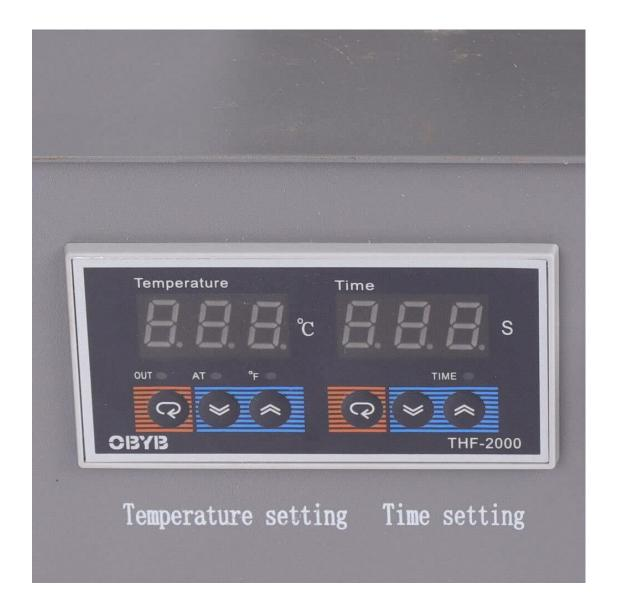
1, Press the "Q" button to set the temperature (the default setting is 287°C). Adjust the temperature using the " $\approx$ " or " $\approx$ " buttons, and press the "Q" button to confirm.
